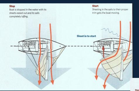
Head up into No-Go Zone to stop To stop the boat head up directly into the No-Go Zone. The sails luft completely and the boat stops. To stop the boat more quickly, a crew member pushes (*backs*) the mainsail against the wind (shown).
